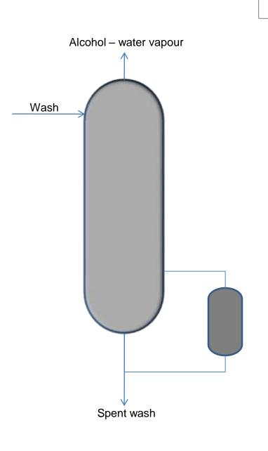
In this column preheated fermented wash is stripped off from all volatile components, including ethyl alcohol.
